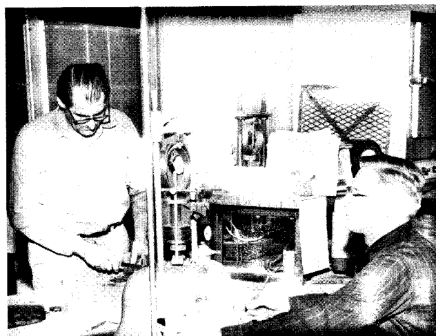
Laboratory unconfined compression tests used to obtain indication of maximum available skin friction for timber piles in clay soil.
